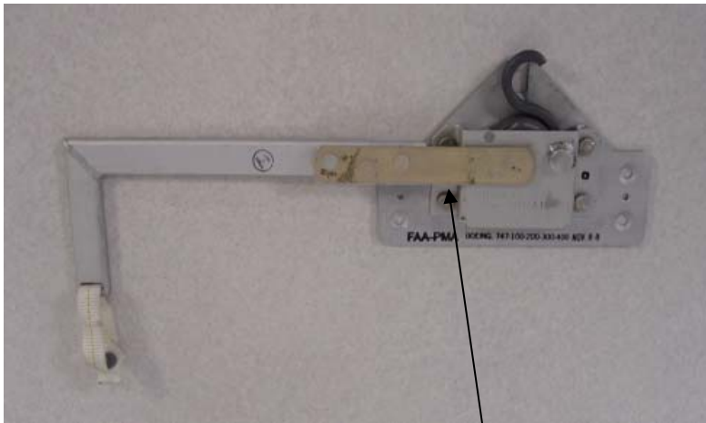
Figure 1. Base Plate to Handle Clearance Measurement Location
