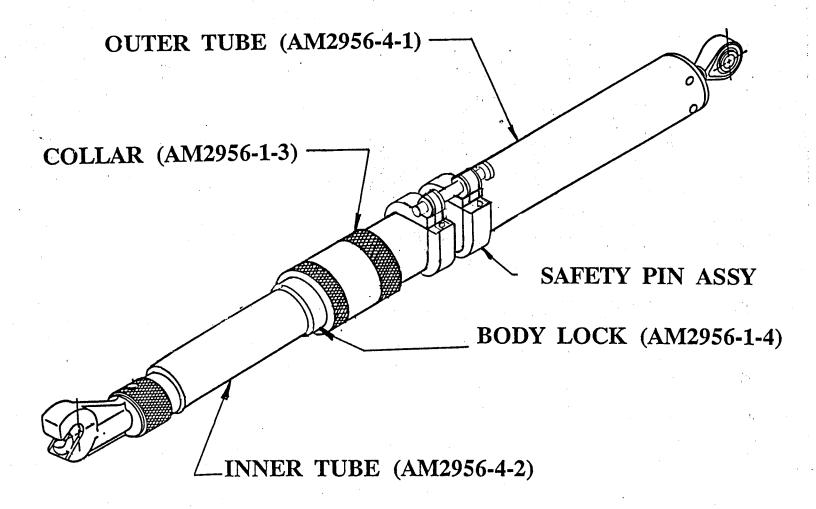
FIGURE 1 - STRUT ASSEMBLY A2956-5A
